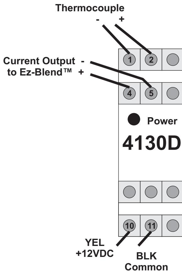
Note: A 250ohm Resistor is required across the Ez-Blend™ Input Terminals.
